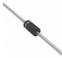
1N5244B_S00Z AMI Semiconductor / ON Semiconductor DIODE ZENER 14V 500MW 5% DO-35
