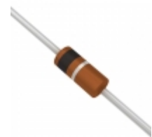
1N5244B-TAP Vishay Semiconductor Diodes Division DIODE ZENER 14V 500MW DO35
