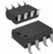
TS190PLTR IXYS Integrated Circuits Division IC RELAY OPTO 150MA 8FLTPK
