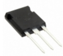
APT43GA90B Microsemi Corporation IGBT 900V 78A 337W TO-247
