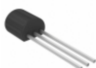
MCP1701A-2502I/TO Microchip Technology IC REG LDO 2.5V 125MA TO92-3
