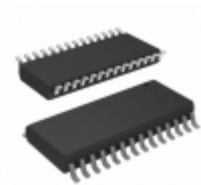
AT28BV64B-25SC Microchip Technology IC EEPROM 64KBIT 250NS 28SOIC
