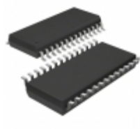
ADM561JRSZ-REEL Analog Devices Inc. IC TXRX RS232 4:5 3.3V LP 28SSOP
