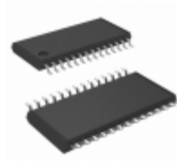
PCA9635PW,112 NXP Semiconductors / Freescale IC LED DRVR LIN DIM 25MA 28TSSOP
