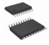
PCA9634PW/S910,118 NXP Semiconductors / Freescale IC LED DRVR LIN DIM 25MA 20TSSOP
