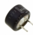
DBN-5R5D224T Elna America CAP 220MF -20% +80% 5.5V T/H
