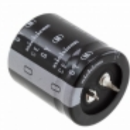
LGY2E471MELB Nichicon CAP ALUM 470UF 20% 250V SNAP
