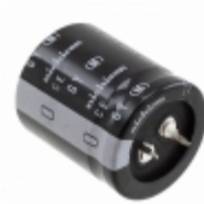
LGY2E561MELB Nichicon CAP ALUM 560UF 20% 250V SNAP
