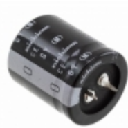
LGY2E471MELB Nichicon CAP ALUM 470UF 20% 250V SNAP
