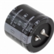
LGY2E471MELC Nichicon CAP ALUM 470UF 20% 250V SNAP
