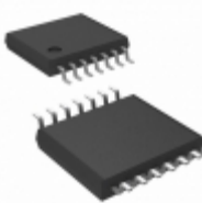
74AC74MTC Fairchild/ON Semiconductor IC D-TYPE POS TRG DUAL 14TSSOP
