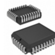
AT49LH004-33JX-T Microchip Technology IC FLASH 4MBIT 33MHZ 32PLCC
