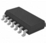
MCP4231T-104E/SL Microchip Technology IC DGTL POT 100K 2CH 14SOIC
