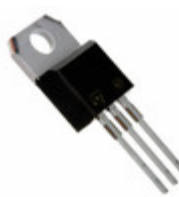
L78M05ABV STMicroelectronics IC REG LDO 5V 0.5A TO220AB
