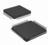
ATXMEGA64C3-ANR Microchip Technology IC MCU 8BIT 64KB FLASH 64TQFP
