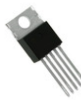
MCP1827-ADJE/AT Microchip Technology IC REG LDO ADJ 1.5A TO220-5
