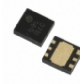
XC6121A528ER-G Torex Semiconductor Ltd IC WATCHDOG TIMER 6-USP
