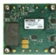
UCH-5/20-D24PB-C Murata Power Solutions Inc. CONV DC/DC 100W 5V 20A
