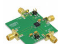
110227-HMC531LP5 Analog Devices Inc. BOARD EVAL HMC531LP5E
