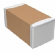
C3216X8R1C335K160AB TDK Corporation CAP CER 3.3UF 16V X8R 1206
