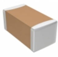
C3216X7T2W683M130AA TDK Corporation CAP CER 0.068UF 450V X7T 1206
