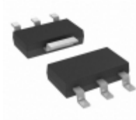
NCP1117STAT3G ON Semiconductor IC REG LDO ADJ 1A SOT223
