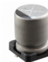
UUA0J331MNL1GS Nichicon CAP ALUM 330UF 20% 6.3V SMD
