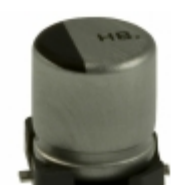
EEV-HB0G101R Panasonic Electronic Components CAP ALUM 100UF 20% 4V SMD
