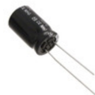
ECA-1EHG222B Panasonic Electronic Components CAP ALUM 2200UF 20% 25V RADIAL
