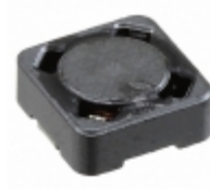
CDRH73NP-471MC-B Sumida Corporation FIXED IND 470UH 240MA 4.18 OHM
