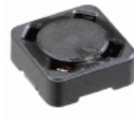
CDRH73NP-681MC-B Sumida Corporation FIXED IND 680UH 190MA 5.73 OHM
