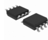
MICRF007YM Microchip Technology IC RECEIVER UHF LOW POWER 8SOIC
