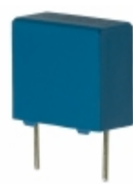
B32912A4473M289 EPCOS (TDK) CAP FILM 0.047UF 20% 440VAC RAD
