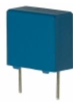
B32912A4563M EPCOS (TDK) CAP FILM 0.056UF 20% 440VAC RAD
