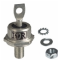
VS-70HFLR60S02 Vishay Semiconductor Diodes Division DIODE GEN PURP 600V 70A DO203AB
