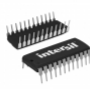
HIN238CPZ Intersil IC 4DRVR/4RCVR RS232 5V 24-DIP
