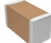
CL31B475KBHVPNE Samsung Electro-Mechanics America, Inc. CAP CER 4.7UF 50V X7R 1206
