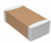
CL31B562KBCNNNC Samsung Electro-Mechanics America, Inc. CAP CER 5600PF 50V X7R 1206
