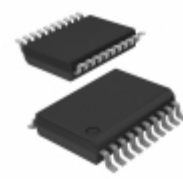
PIC32MM0032GPL020T-I/SS Microchip Technology IC MCU 32BIT 32KB FLASH 20SSOP
