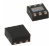
MIC5321-OGYMT-TR Microchip Technology IC REG LDO 2.9V/1.8V 0.15A 6TMLF
