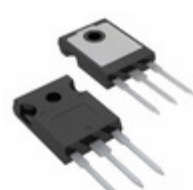
IRG4PH40KDPBF Infineon Technologies IGBT 1200V 30A 160W TO247AC
