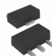
MCP1804T-3002I/MB Microchip Technology IC REG LDO 3V 0.15A SOT89-3
