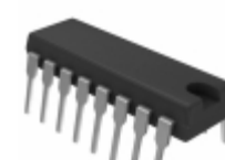
MAX712EPE+ Maxim Integrated IC CNTRLR NICD/NIMH 16-DIP
