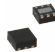
MIC5335-KDYMT-TR Microchip Technology IC REG LDO 2.6V/1.85V 0.3A 6TMLF
