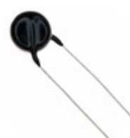
ERZ-V14D751 Panasonic Electronic Components VARISTOR 750V 5KA DISC 14MM
