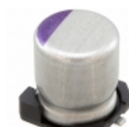
6SVP82M Panasonic CAP ALUM POLY 82UF 20% 6.3V SMD
