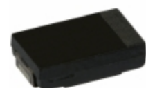
EEF-SX0E391XE Panasonic Electronic Components CAP ALUM POLY 390UF 20% 2.5V SMD
