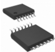
74HC27PW,112 Nexperia USA Inc. IC GATE NOR 3CH 3-INP 14-TSSOP
