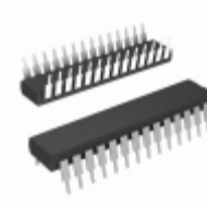
PIC24FJ32GB002-I/SP Microchip Technology IC MCU 16BIT 32KB FLASH 28SDIP
