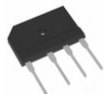
TS10P05G C2G TSC (Taiwan Semiconductor) BRIDGE RECT 1P 600V 10A TS-6P
