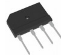
TS10P05GHD2G TSC (Taiwan Semiconductor) BRIDGE RECT 1P 600V 10A TS-6P
