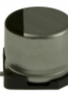
EEV-HA1C470P Panasonic Electronic Components CAP ALUM 47UF 20% 16V SMD
