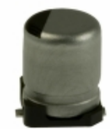
EEV-HA1C100R Panasonic Electronic Components CAP ALUM 10UF 20% 16V SMD
