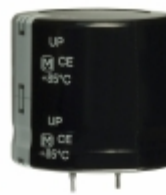
ECO-S2HP181EA Panasonic Electronic Components CAP ALUM 180UF 20% 500V SNAP
