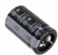
LGY1E123MELA40 Nichicon CAP ALUM 12000UF 20% 25V SNAP
