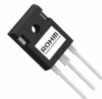
RGW80TS65DGC11 LAPIS Semiconductor 650V 40A FIELD STOP TRENCH IGBT
