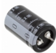
LGX2D471MELZ35 Nichicon CAP ALUM 470UF 20% 200V SNAP
