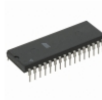
AT29C020-15PC Microchip Technology IC FLASH 2MBIT 150NS 32DIP
