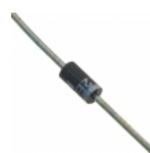
3EZ18D5/TR12 Microsemi Corporation DIODE ZENER 18V 3W DO204AL
