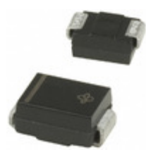
SMBJ7.0-E3/5B Vishay Semiconductor Diodes Division TVS DIODE 7VWM 13.3VC SMB
