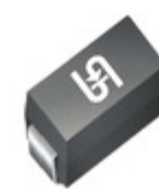
SMAJ14CA M2G TSC (Taiwan Semiconductor) TVS DIODE 14V 23.2V DO214AC
